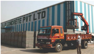
Loading: High powered truck mounted cranes facilitate delivery of strapped blocks at the sites
